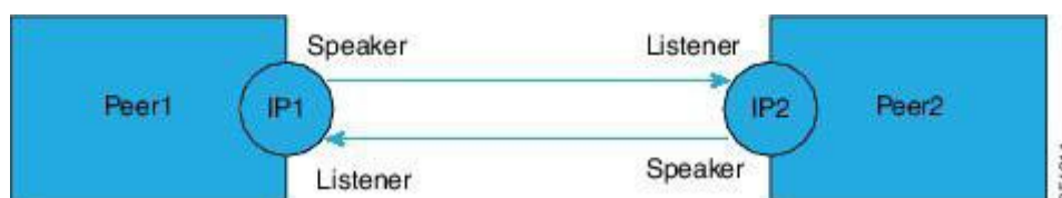
Figure 17: Bidirectional SXP Connection
