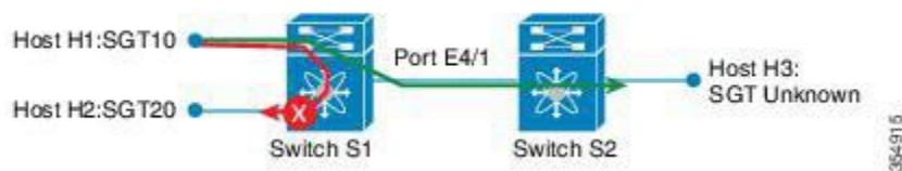
Figure 14 : SGACL Policy Enforcement Per Interface Disabled
